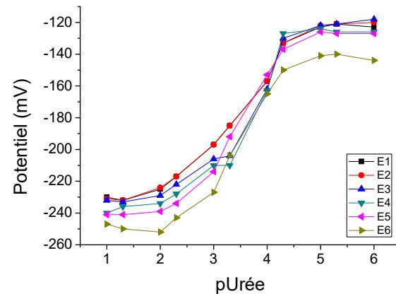
Influence of the enzyme immobilization method on the sensitivity and stability in time of the biosensor.
