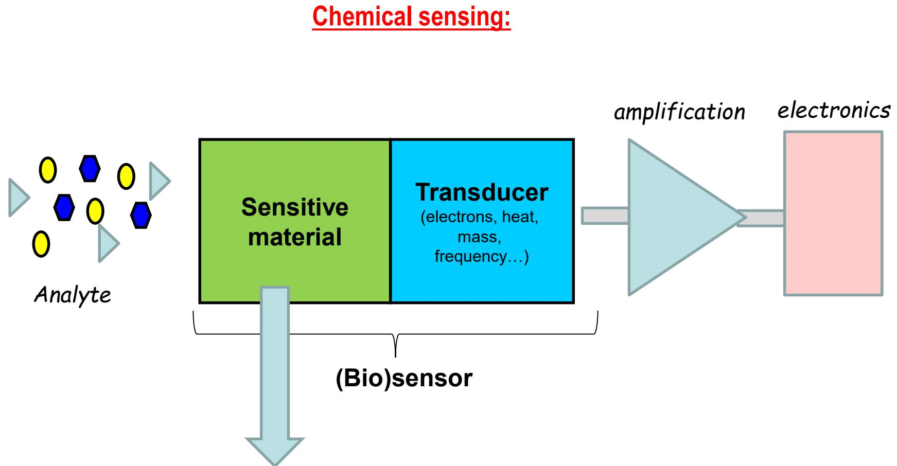
A large number of sensitive materials exist: oxide particles, carbon materials (graphene, CNT), organic materials, polymers (electrodeposited, self-assembled, molecular imprinted)
